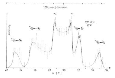
Fig. 2. Plot of the observed <sup>67</sup>Zn spin echo profile at a constant frequency of 7.81 MHz in zinc metal.
