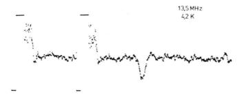
Fig. 1. Single scan of a 90°-τ-180° spin echo pulse sequence at 5.0172 T of <sup>67</sup>Zn in zinc metal.
